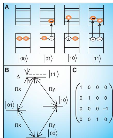
**Fig. 1.** (A) Two exciton transitions in a single QD. (B) Excitation-level diagram, where  $|00\rangle$ ,  $|01\rangle$  and  $|10\rangle$ , and  $|11\rangle$  denote the ground state, the excitons, and the biexciton, respectively. The optical selection rules for various transitions are labeled.  $\Pi_x$  and  $\Pi_y$  indicate orthogonally and linearly polarized lights.  $\Delta$  represents the binding energy. (C) The transformation matrix for a CROT gate.
